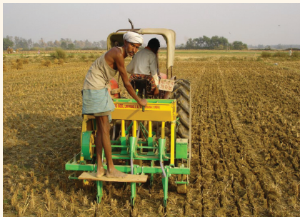
Seeding by Zero-tillage seed drill
